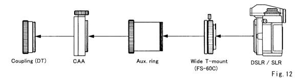
◆ Astrophotography with the Flattener By using the dedicated flattener with the connection shown below, you can take flat field astrophotos. See the system chart for connection.
