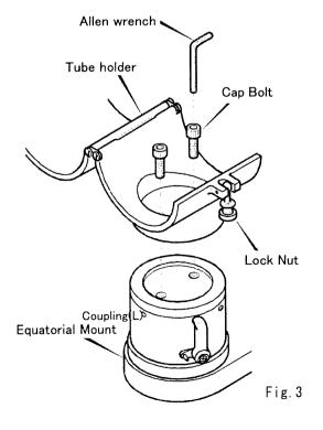
The correct way to attach the tube holder to the mount is to use the two cap bolts provided. After an optical tube has been set into the tube holder, the next step is balancing. Refer to Fig.4.
